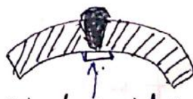
Single welded butt joint with backing strip
